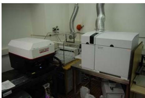
System of laser ablation ICP-MS at the Laboratoire Archéoscience (Rennes)
